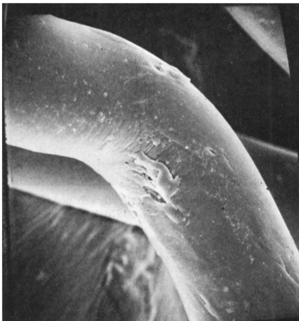
Fig. 7. SEM micrograph of the tensile and compression damage in a highly crimped polyester fiber, 935 \times .
