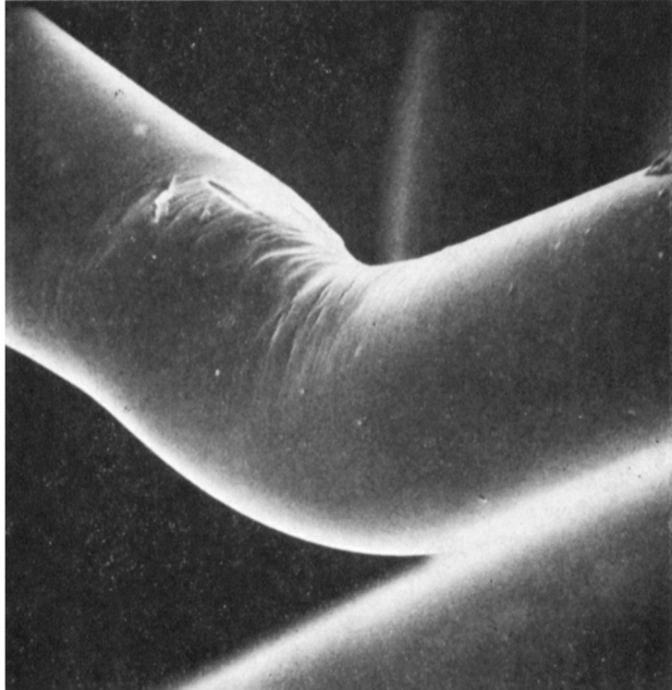
Fig. 6. SEM micrograph of the compression damage in moderately crimped polyester fiber, 470 \times .
