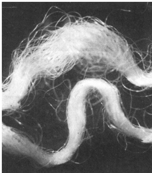
Fig. 1. Photomicrograph of crimped and uncrimped polyester fiber, 40 \times .
